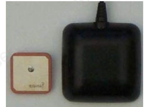
GPS antenna 25 mm x 25 mm x 4 mm
