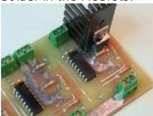
7. Test it with a 1 KOhm resistor in series with the power supply. This will provide enough current to light an LED, but not enough to blow up a MOSfet.
